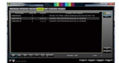
7. Click the tab of "DMX devices", set port status to "ON" if connected successfully. Now, you can use computer to control lamps via ArtNet-DMX-8S.
